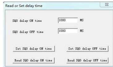
Input SQ0 Delay ON time Click "Read SQ0 delay ON time" and input correct password to download Delay ON time to SMS module.
