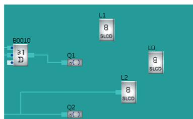
The function block L0 displays the set value and the running value of time delay relay.
