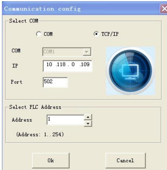
When it is correctly linked, this interface disappears automatically, and you can enter into the main interface of APB Soft. If it fails to connect, the following information will be given. And you should check if the IP address and port number are written accurately; if the cable connection is reliable and the power linkage is proper.
