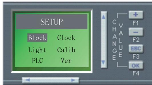
On this interface, move the cursor position with “← → ↑ ↓” keys. Select the block parameter (Block), clock parameter (Clock), PLC address (PLC) and version number (Ver), and press “OK” key to confirm. Then press ESC to return the main interface.
