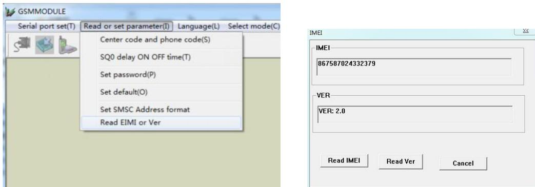
IMEI (international mobile equipment identity) is a symbol to distinguish the mobile equipment, each SMS module is assigned a unique and different IMEI.
