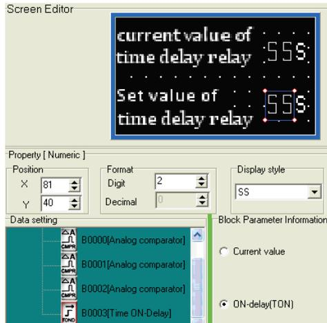
3. Create a screen page for “Display the current value of pressure sensor P1 and the set value of analog comparator”.
