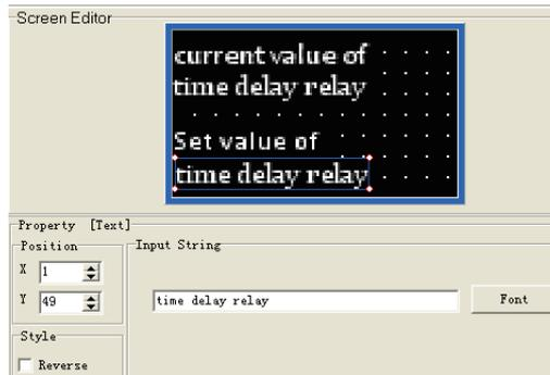
Choose the component "B", and select "Function block B0003 (ON-delay). The "current value" is chosen as the parameter. Displayed digits: 2; decimal digits: 0
