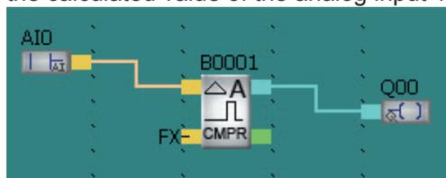
Input 1 is connected to AI0;
