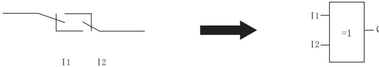
When the status of inputs is different, the output status of XOR is 1.
