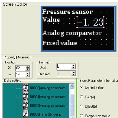
Choose the component “**B**”, and select “Function block B0000 (universal analog comparator).The “Running value of the block” is chosen as the parameter. Displayed digits: 3; decimal digits: 2.
