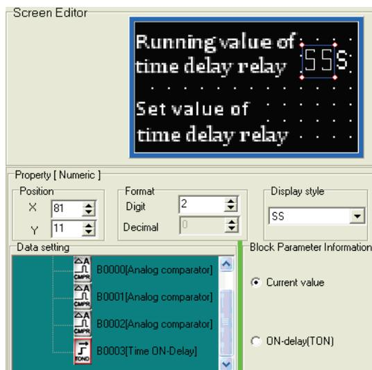
Choose the component "B", and select "Function block B0003 (on-delay). The "ON-delay" is chosen as the parameter. Displayed digits: 2; decimal digits: 0.
