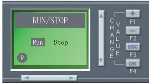
On this interface, change the cursor position by moving “← →” key. Select “Run” or “Stop” and press “OK” key to confirm. Press ESC to return to the main interface.
