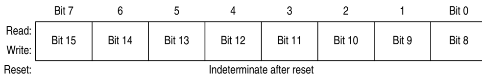
Figure 16-14. TIM1 Channel x Register High (T1CHxH)
