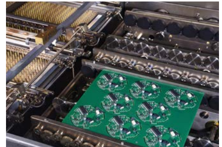
The Erska EXOS 10/26 has a 4-part transport system which is lubricant-free in the vacuum module.
